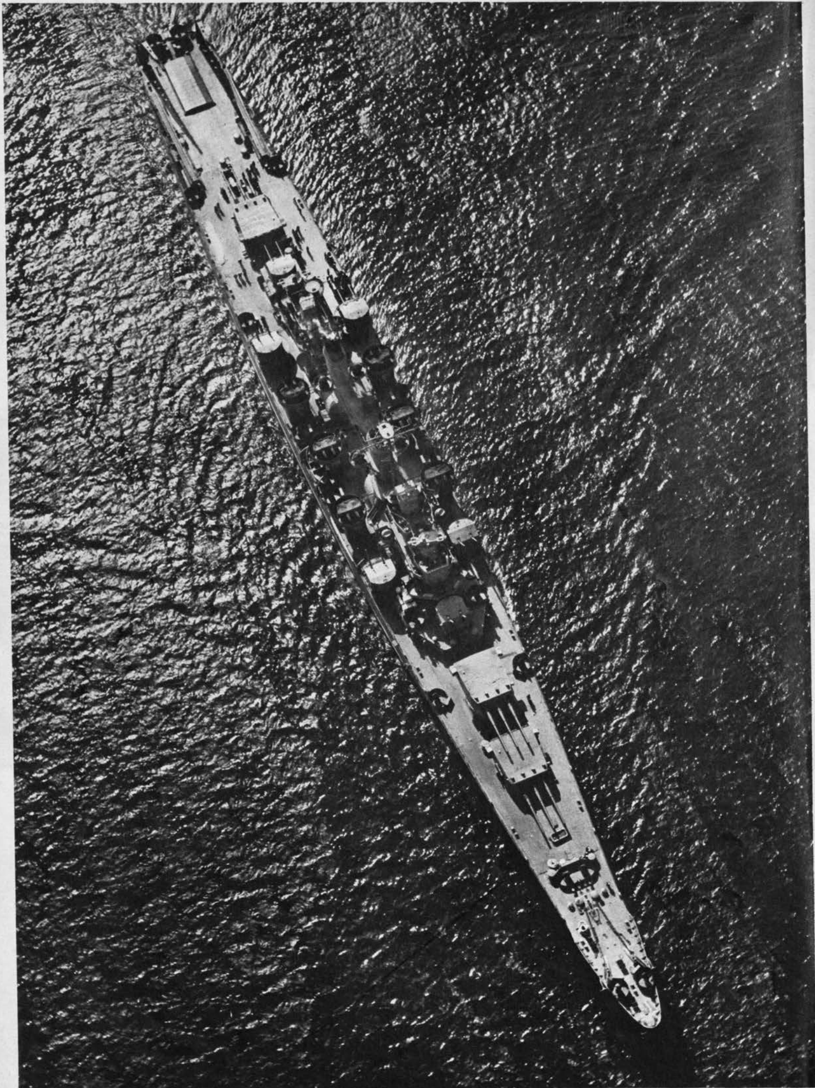
Seen from above, the U.S.S. Baltimore bristles with anti-aircraft in twin mounts. Nine 8-in. guns in two triple turrets forward and one
